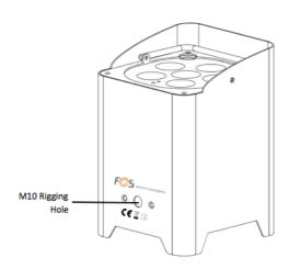
When install the fixture to crossbar or truss, always use an extra safety cord (not supplied with the fixture). Users also need to make sure the crossbar is stable or not moving, and can support a weight of 37 kg (fixture net weight 3.7kg).
